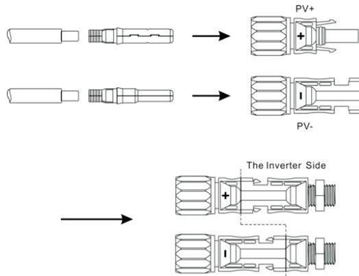
Similar to the traditional inverter connecting, the input of PV panel energy can be realized by using MC4 PV terminal, the detail steps are as follows :
