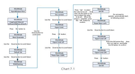
Under the permission given by your energy provider, the ratio of your system output power divided by the rated power of the inverter is called Export Limit Rate. For instance, if the energy provider only accepts 4kW from your 5kW system, then the Export Limit Rate of 5kW inverter is 80.0%.
