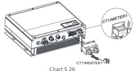
1.Meter and CT can't be installed at same time, please set the sensor model when selecting CT or electricity meter, please refer to section 6.3.3 for details.
