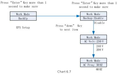
In the back up you can set EPS, including enable or disable (default is enable), AC voltage(default is 230V) and frequency (default site 50HZ).
