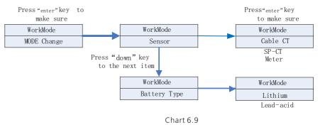
The MODE change has two options what are sensor and battery type, sensor is cable CT (default), meter and SP-CT(wireless RF transfer). In the battery type, you can choose lithium battery or lead-acid battery.
